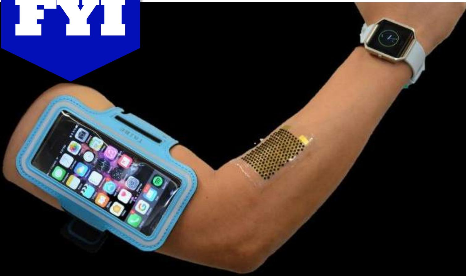
A team of engineers has developed stretchable fuel cells that extract energy from sweat and are capable of powering electronics, such as LEDs and Bluetooth radios. The biofuel cells generate 10 times more power per surface area than any existing wearable biofuel cells. The devices could be used to power a range of wearable devices.
